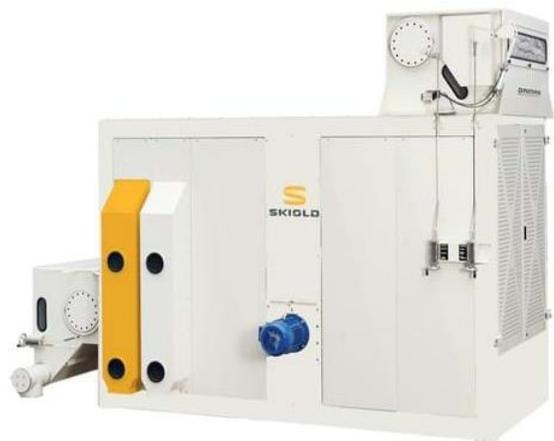
The Hotyp Indented Cylinders are hollow shells and layered with small indents that match the optimal size of the grain or seed running through the machine. The spinning force of the cylinder forces the grain or seed of near-perfect optimal size and shape into the indents. This highest quality product then travels through this cylinder completing the sorting and the sizing ensuring Purely Canada product is of only the highest standard when it reaches its end consumer.
